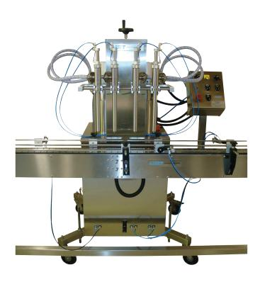
The Asset AMF-4C is a versatile completely automatic four head filling machine designed to fill liquids, creams and pastes of varying volumes. The AMF-4C provides simple user operation with high levels of output & reliability.
