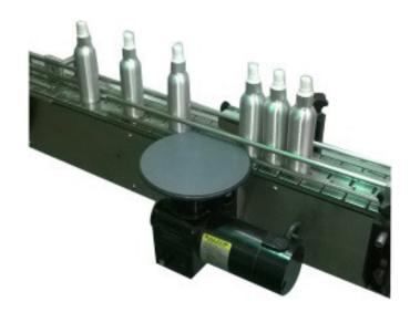
The Asset ASW-10 spacing wheel is an adjustable container handling accessory that can be mounted to a conveyor. The unit spaces out product containers to a pre-determined width on the conveyor system in prearation for other processes such as filling, capping batch coding etc. Powered by standard 240v 10 Amp power, the spacing wheel has a variable speed controller & comes with custom parts for special applications.
