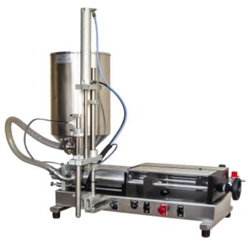
The AV-3-BUF SIngle Head Volumetric Liquid Filler offers a simple to operate, heavy duty design with a proven history of reliability and ease of use and cleaning. With a fill process that begin at the bottom of the container this filler is designed to be used with bubbling or foaming liquids that aren't suitable for standard fillers. This filler comes standard with a positive shut off nozzle. Ideal use with all creams, pastes, and liquids.
