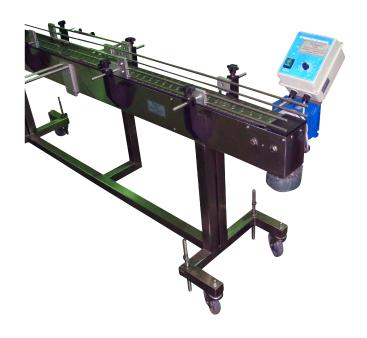
The Asset CV-6 Slat Conveyor range provide versatile solutions to suit most motion requirements. Powered by standard 240v household power, the CV-6 is available in 1.2, 2.4, 3.6 & 4.8 metre options, & comes with various accessories to suit most configurations.
