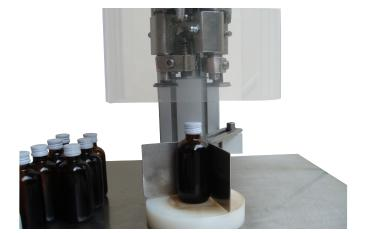
The ROPP-T capper is a versatile semi-automatic capping machine designed for all non-threaded aluminium caps. The ROPP-T provides simple user operation with high levels of performance & reliability.
