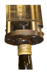
The ROPP-TM capper is a versatile semi-automatic capping machine designed for all non-threaded aluminium caps. The ROPP-TM provides simple user operation with high levels of performance & reliability.
