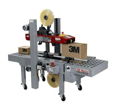
The 3m-Matic-200a Case Sealer is an adjustable bottom belt drive case sealer, designed to seal the top & bottom centre seams with consistent & durable case taping. The solution is simple to configure with manual adjustments for multiple box sizes. The durable bottom belt drive offers dependability for cases weighing up to 40 Kilos.
